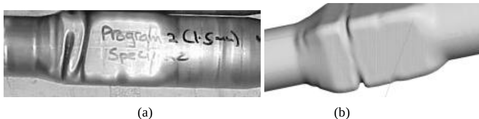
Figure A- 16: Sample hydroformed tube with LP2, t_0 = 1.5 mm, mat. A; (a) actual wrinkle shape and (b) FEM result;
