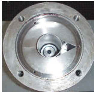
Figure I-81: Pear-shaped tooling for lubrication tests in the expansion zone.
