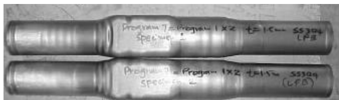
Figure A- 13: Hydroformed samples with LP 7, t_0 = 1.5 mm, mat. A.
