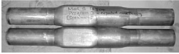
Figure A- 8: Hydroformed samples with LP 3, material B
