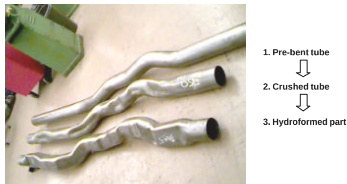
Figure I- 35: Automotive tubular parts formed at intermediate stages
