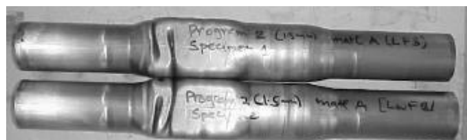
Figure A- 11: Hydroformed samples with LP 2, t_0 = 1.5 mm, mat. A.
