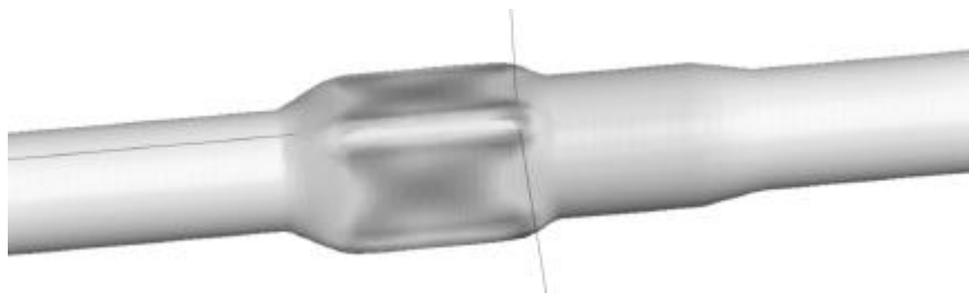
Figure II- 25: geometry obtained by adaptive FEM simulation of the LP given in Figure II- 23. Different tones of gray indicate different thickness values.
