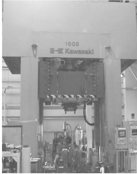
Figure A- 4: The Hydroforming press located at the Kawasaki HydroMechanics plant in Japan.
