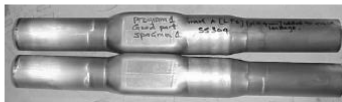
Figure A- 10: Hydroformed samples with LP 1.2, t_0 = 1.5 mm, mat. A.
