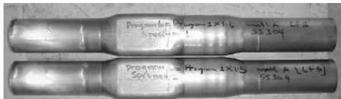
Figure A- 12: Hydroformed samples with LP 6, t_0 = 1.5 mm, mat. A.
