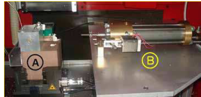
2. Overview of the micro QSD placed in the Kern EVO machining centre [A = tool holder block, B = percussion system].
