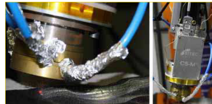
3. Developed new cladding head on the left and a detail of the cladding nozzle on the right.
