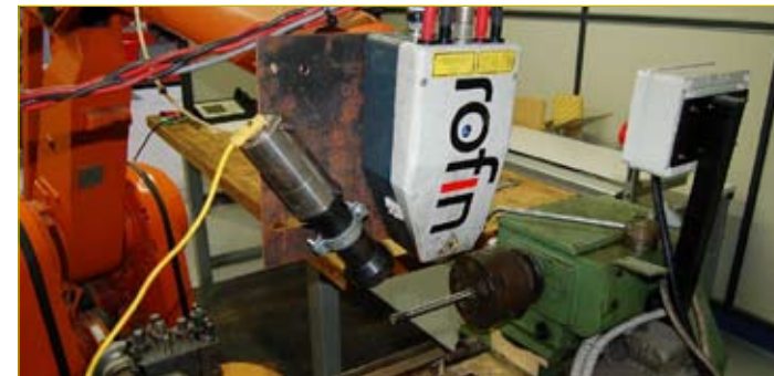
2. Setup of the Apparent Spot laser hardening system
